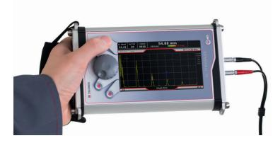
The SONOWALL 70 can be used in two operating modes - wall thickness mode and flaw detector mode. Both software modes can easily be updated vice versa and include:
