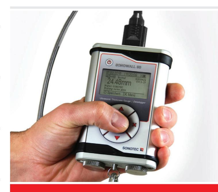
**ULTRASONIC WALL THICKNESS GAUGE**
