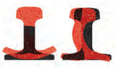
Figure 1 - Example of guided wave mode shapes with energy concentrated in the foot (left) and web (right) of the rail respectively.
