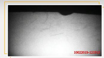
OpenVision is a true nondestructive testing (NDT) method that uses live video output for real-time radiographic inspection of hundreds of feet (many tens of meters) of insulated piping for indications of corrosion.
